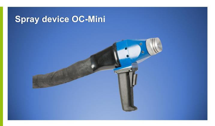
The spray device OC1 with the closed nozzle system is specialized in the processing of corrosion protection wires. The special geometry of the nozzle system components allows a very fine atomization of the melt particles, whereby a correspondingly fine coating with low surface roughness is achieved. This provides a significant savings potential of paint for subsequent topcoats.
